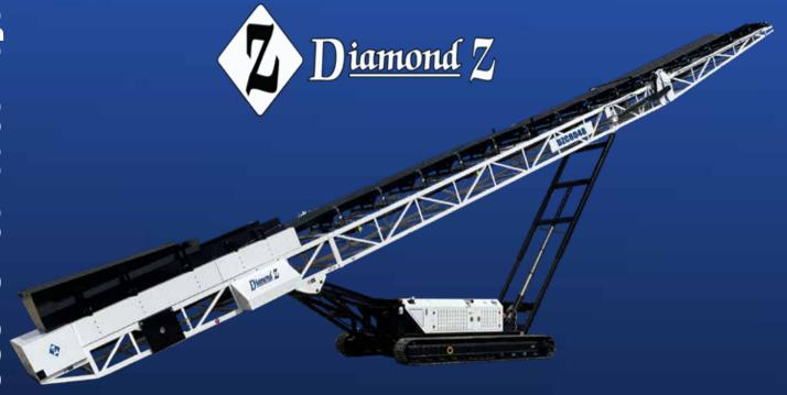
Take your material processing to new heights with the DZC8048T Tracked Stacking Conveyor. A full 80' in length with a 48" wide belt and variable height adjustment, this stacker allows your Dlamond Z Grinder to keep humming!
