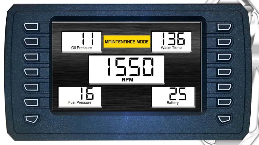
Maintenance mode is enabled when tub/crush roller are hydraulically pin in the safe maintenance position.
