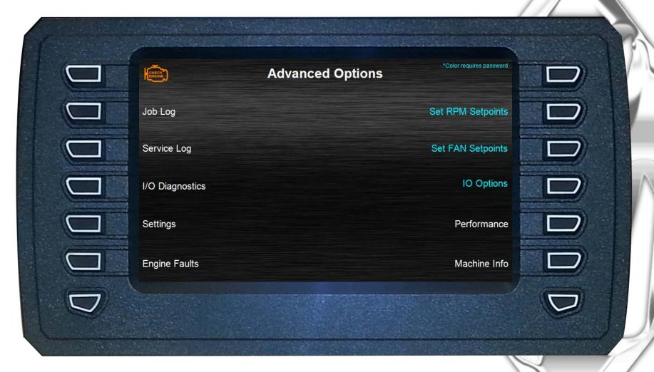
Advanced options screen is how to check engine fault code, service log, IO diagnostic inputs & outputs, machine setting, setting the RPM set points, setting the fan purge set points, machine performance
