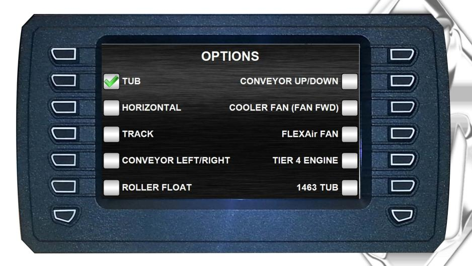
This set up screen allows you to configure your plc for any Rule Steel/Diamond Z product without the necessity of having to reprogram or inventory multiple plc's.
