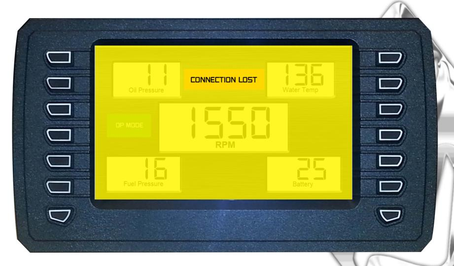
Digital Screen will flash every 2sec showing Data Connection Lost: Will need to check the Data link coming to the screen? The machine will function with Data Connection lost.
