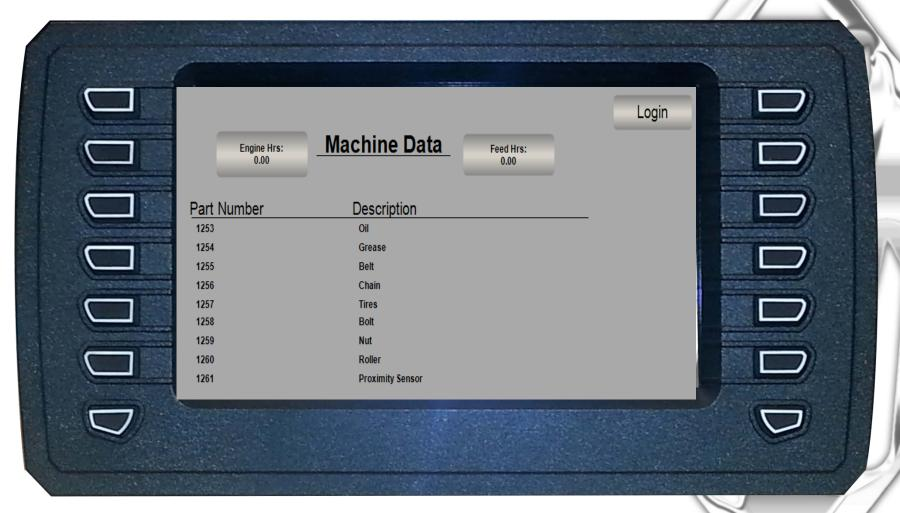
You can store specific machine data such Belt length, filter part numbers, air filters etc.
