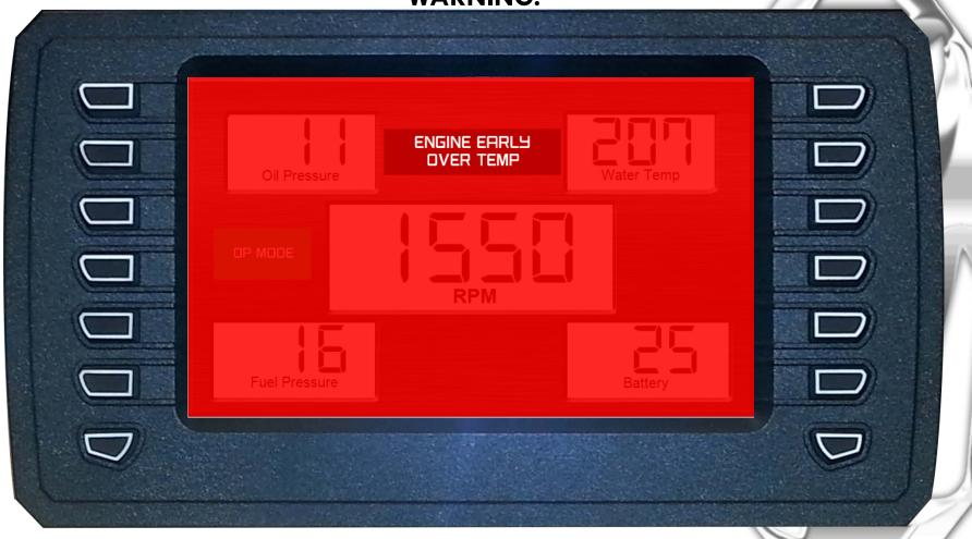
DIGITAL SCREEN WILL FLASH RED EVERY 2 SEC. WHEN THE FLUID COUPLER TEMP EXCEEDS 180\*F. THIS WILL SHUT OFF THE FLUID COUPLER AND IDLE THE ENGINE DOWN.
