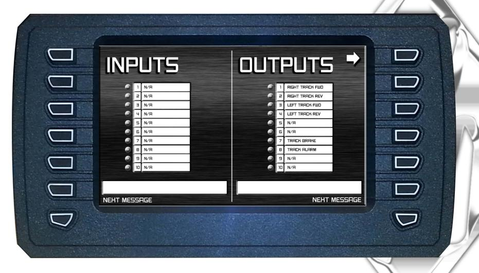
Any active faults can be reset by turning off battery disconnect key for 30 seconds
