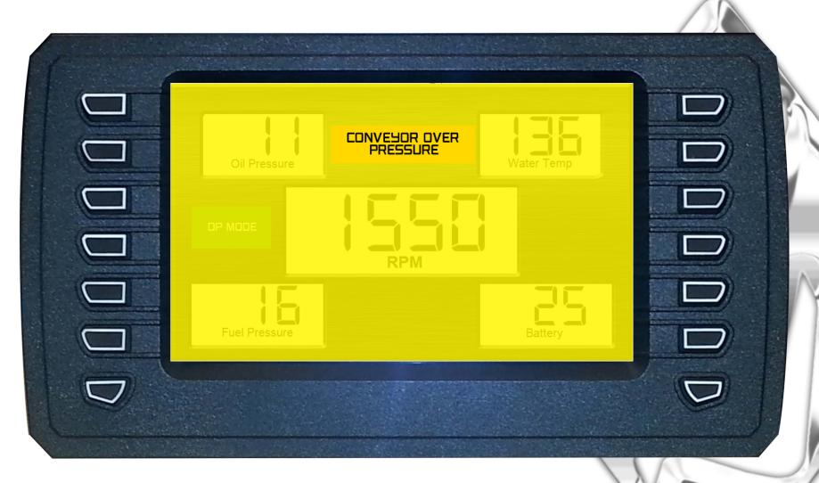
Digital Screen flashes every 2sec Showing Conveyor Over Pressure: This Will Shut the Feed System OFF. After the Conveyor Pressure Drops be low 1800psi the screen will go back to Normal and Feed will resume.
