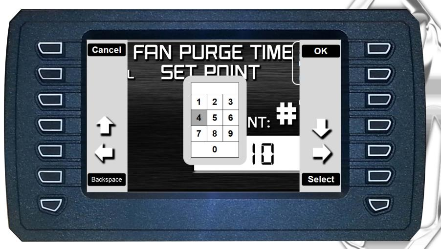
To change the fan purge setting enter the desired time setting on the keypad
