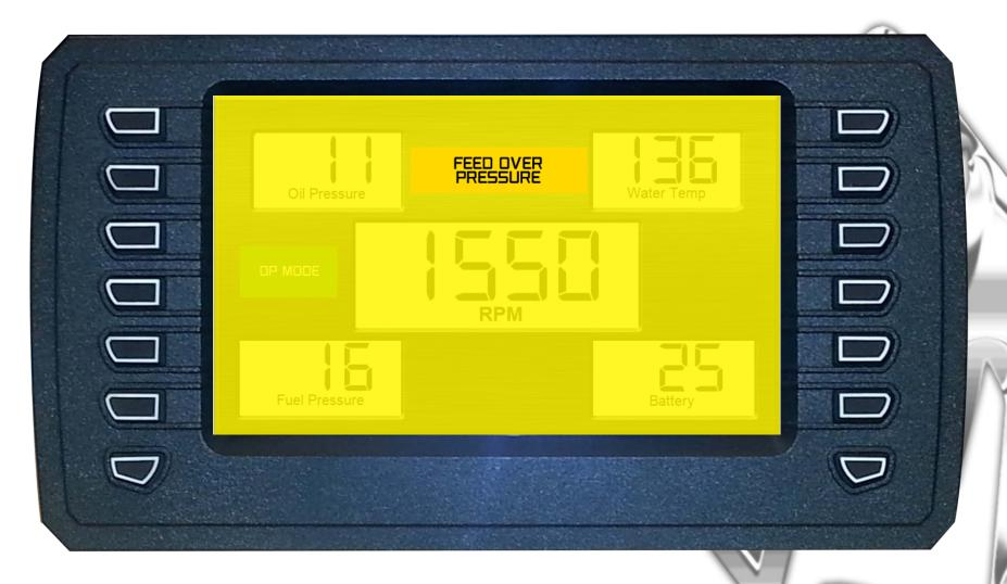
This Screen Flashes ever 2sec while the feed system is over pressure. (TUB)After 3.5sec the feed system will auto reverse for 2.5sec. Then go back forward. (DZH) After 2sec the feed will auto reverse for 1sec.
