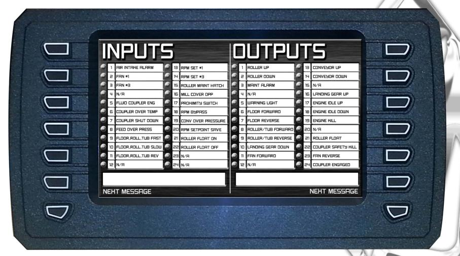
This Input/Output screen is reached by selecting I/O diagnostics screen in the advanced options screen. With normal functionality when a sensor input is activated the corresponding light will lite green. If there is abnormal activity such as a dead short or over amp situation it will show yellow and scroll the fault code below.
