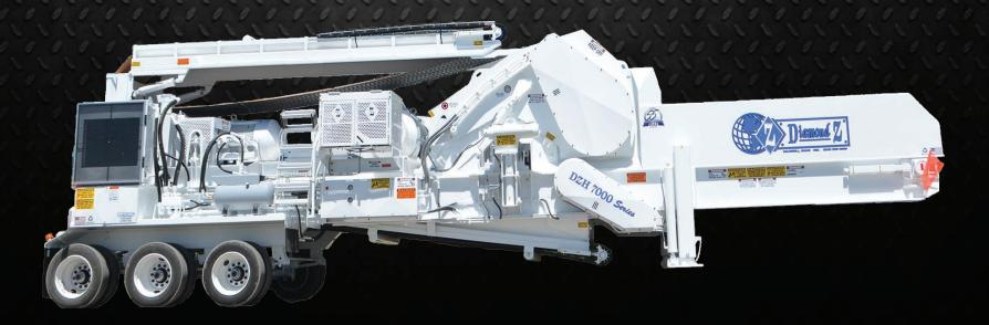
Diamond Z mobile electric grinders house Teco Westinghouse mill drive motors, Teco Westinghouse hydraulic drive motors and a 480 V single soft start control system. These mobile mounting systems create ease of transportation and increases resale value. Diamond Z Electric grinders pack all the punch you expect from a Diamond Z, in an environmentally friendly electric option.
